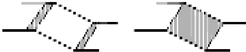
Figure 3.D.6 Markings on an internal ramp
